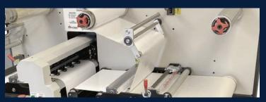
No added costs, no added waiting. IntoPrint's RF1430 digital finishing system is a roll-to-roll converting system that laminates, cuts, strips and slits your labels in one pass and cuts any custom shape on-demand. The RF1430 uses the same digital vector files that you would normally send to your flexible die suppliers. Our technology will make you more profitable, and more competitive, when it comes to delivering shorter runs and customization to your customers.
